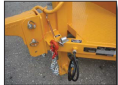
Adjustable, 4 position pintle hitch with safety chains and electrical breakaway switch to engage trailer brakes in case of hitch disengagement.
